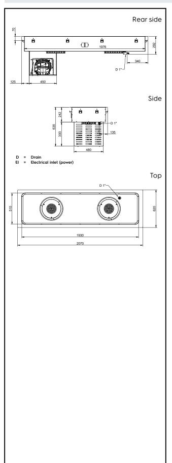
$\qquad \qquad \text{Drop-In} \\ \text{Drop-in refrigerated well, static with fan (6 GN container capacity)}$
