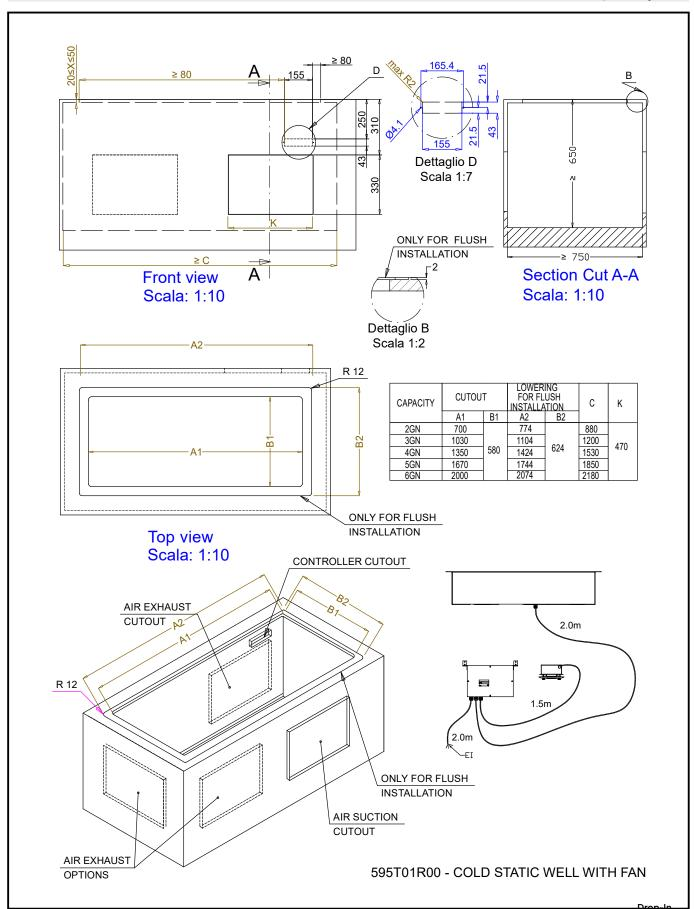
Drop-in refrigerated well, static with fan (6 GN container capacity)
